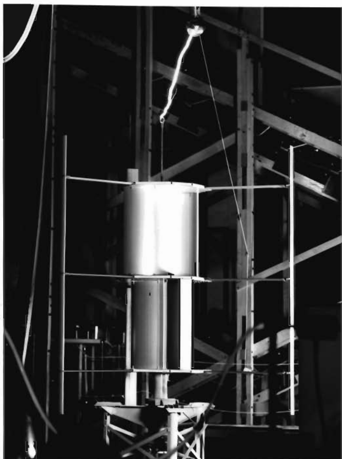
Fig. 5 The ERIGEN turbine in lightning-strike-test in a high voltage laboratory.
