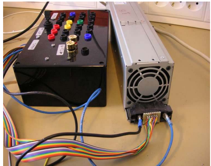
Fig. 8. “Server simulator” for testing of embedded power units
